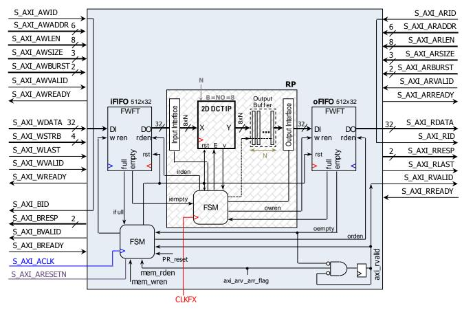
■ The input and output of the 2D DCT IP require more than 32 bits when N = 8, 16. This requires an Input interface to the iFIFO and an Output interface to the oFIFO. The figure shows the different interfaces for each N (4, 8, 16) when B=NO=8. As the FSM @ CLK\_FX controls data flow from the input and the output, it depends on N.
